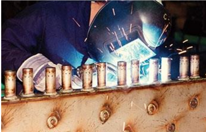
Figure 55. Gas Metal Arc Welding (MIG)
