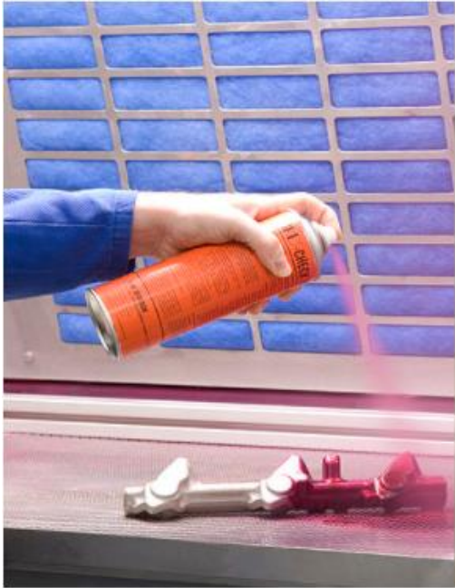
Figure 85. Penetrant Testing Application
