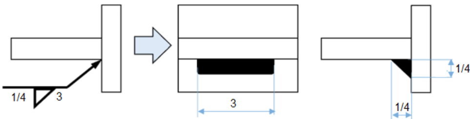
Figure 38.1/4-inch fillet weld with a length of 3 placed on the arrow side
