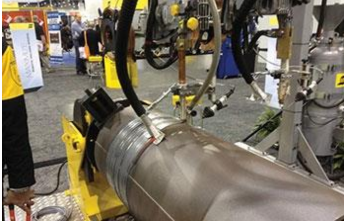
Figure 53. Submerged Arc Welding (Sub-Arc)
