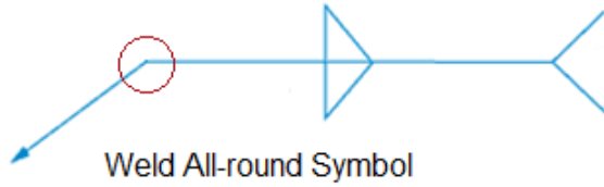
Figure 33. Weld All-round Symbol
