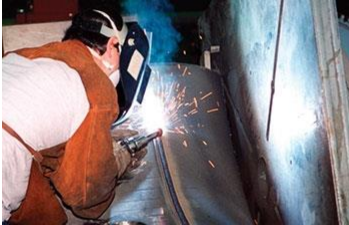
Figure 54. Flux-Cored Arc Welding (Flux-Cored)
