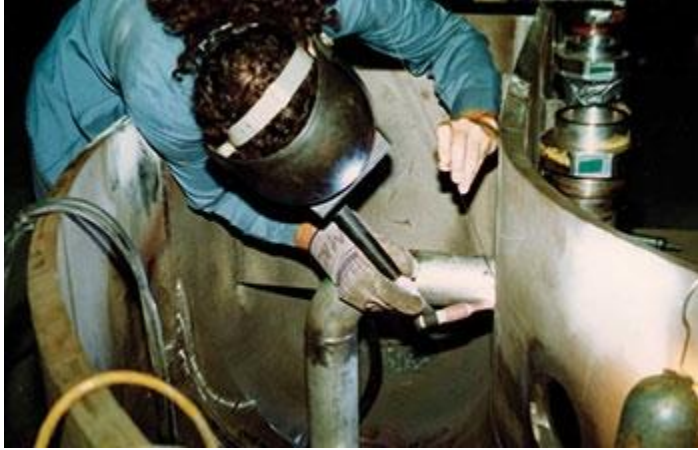
Figure 56. Gas Tungsten Arc Welding (TIG)
