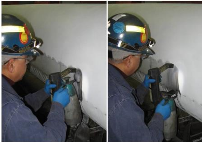
Figure 87. Magnetic Particle Testing of a Pipeline
