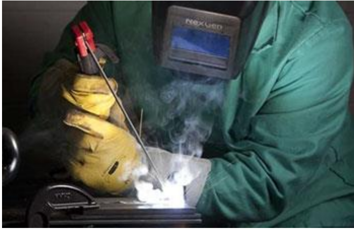
Figure 52. Shielded Metal Arc Welding (Stick)
